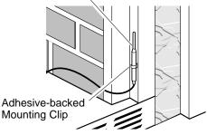
Figure 34 - Locating Thermostat Sensing Bulb on Factory-built Metal Fireplace
